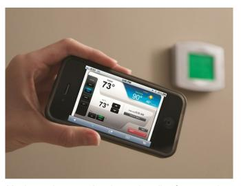
Monitor and set your heating and cooling from anywhere in the world with a Wi-Fi enabled thermostat, which can also reduce energy use.
