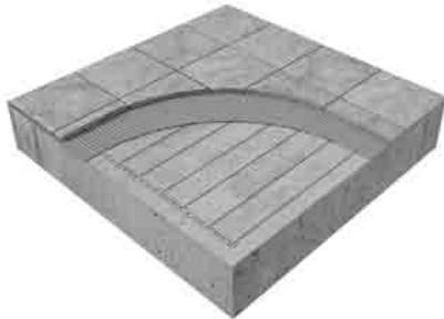
Infloor Electric Cable over concrete slab.
