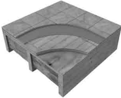
Infloor Electric Cable over wood frame floor with double plywood
