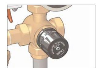
4) Open the shut-off valves again and set the mixing valve at the temperature desired.
