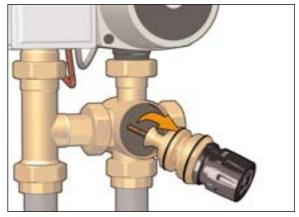
**3**) Replacement cartridges come complete with adjustment knobs.
