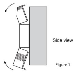
The Front Upper cover can be removed to access the mounting holes or the fuse.
