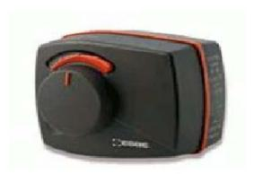
30006 is a rotary motion, non-spring return actuator. It is used specifically with ESBE mixing valves in sizes ½" to 2". The 30006 has a manual override as standard. Mounting hardware for the mixing valve comes with the actuator. A model with one auxiliary switch is also available.
