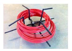
Item 13 pull on tubing to begin installing tubing, the tube uncoiler will rotate to allow tubing to be uncoiled
