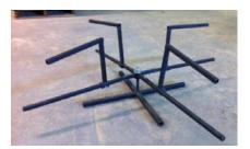
Item 11 Remove L braces and put roll of tubing onto uncoiler
