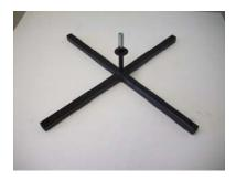
Item 2 Install washer on the base of the uncoiler
