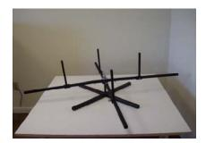
Item 10 Install L braces onto the vertical assemblies L braces should face out. Tubing uncoiler is completely assembled
