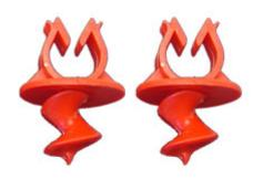
Screw Clip is used for attaching either 3/8" or  $\frac{1}{2}$ " tubing to polystyrene insulation. Insulation minimum thickness is 1". Can be used with Foam Tube Clip tool part # 26016
