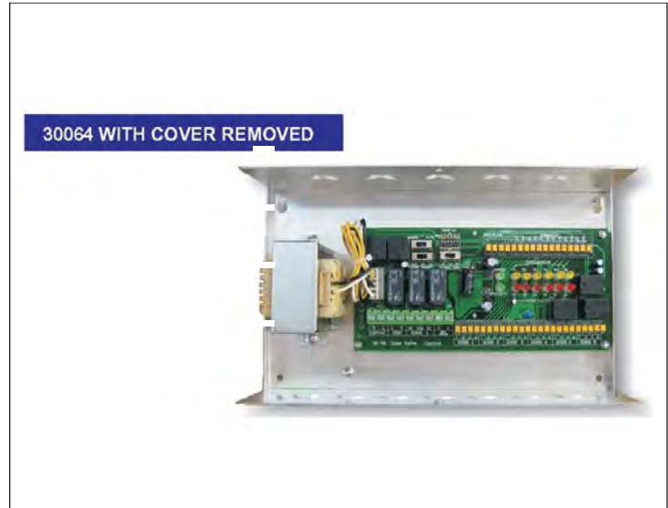
30064 shown below with transformer
